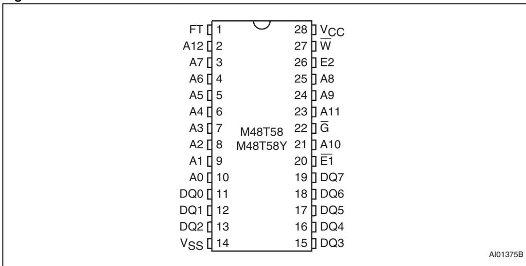
**Figure 3. SOIC connections**
