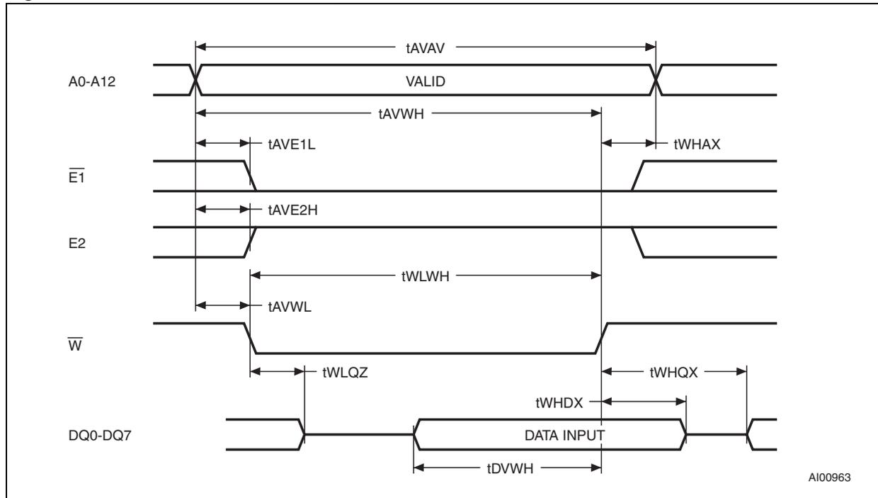
Figure 7. Chip enable controlled, WRITE AC waveforms
