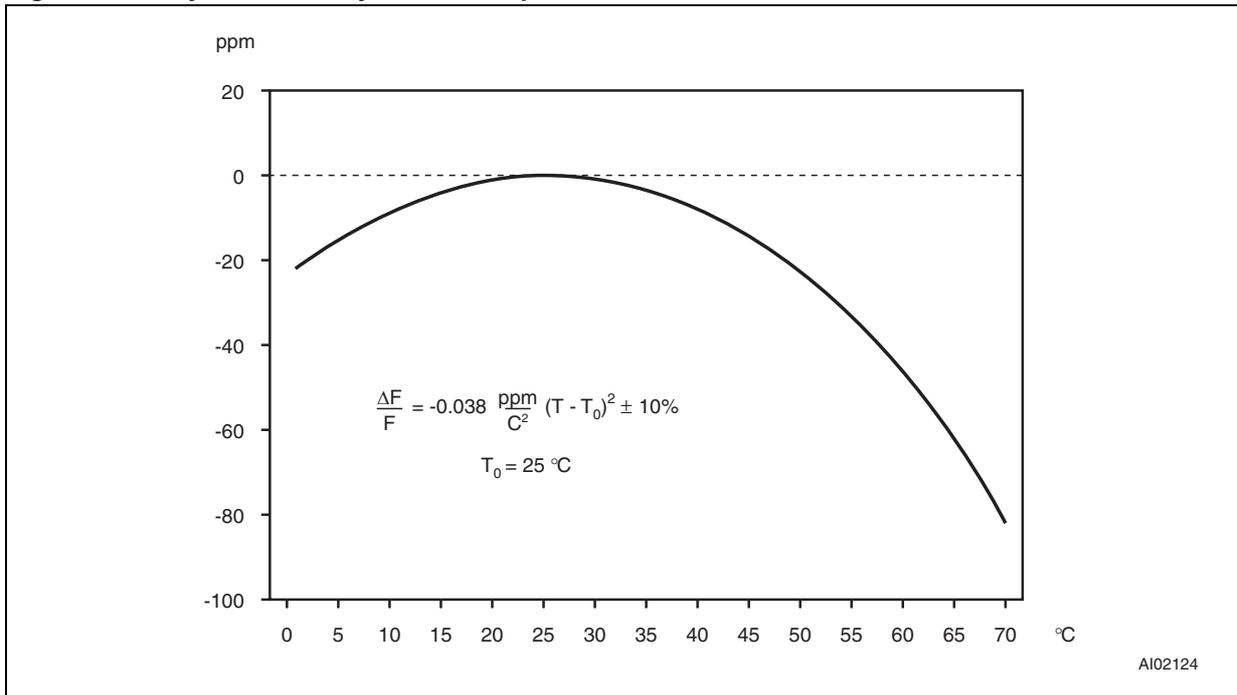
Figure 9. Clock calibration
