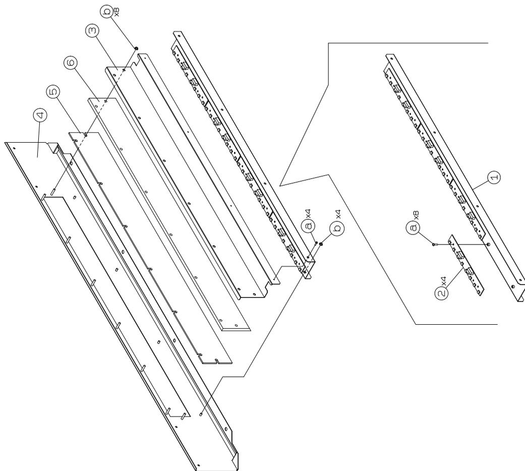
Fig. 58 ASS'Y, STAGE BOARD
