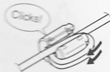
Wind the cable two turns around the clamp filter.
