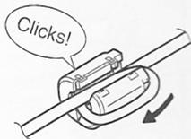
Wind the cable one turn around the clamp filter.
