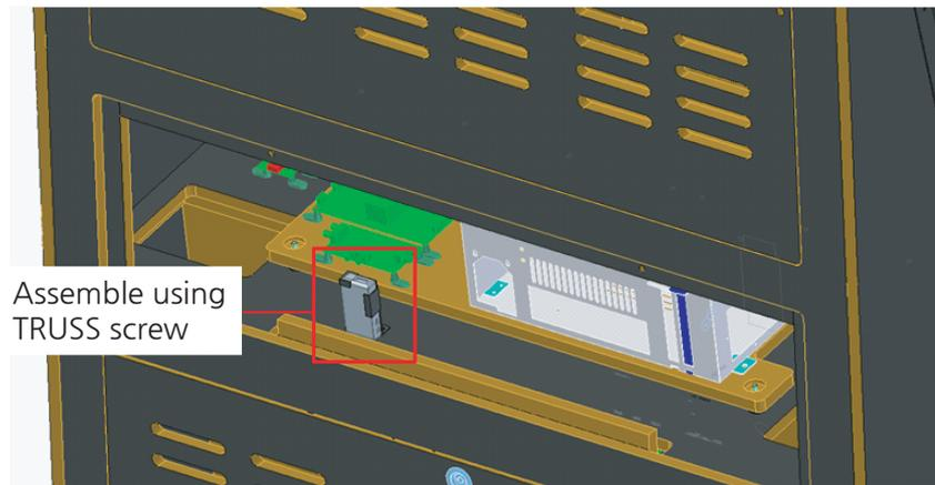
Assemble using TRUSS screw
