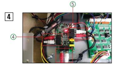
Slightly lift up front side of PC BASE COVER, detach 4 SPEAKER WIRE [6EA] and 5 POWER WIRE.
